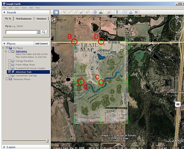
Before closing the New Image Overlay dialog box, you need to adjust (georeference) the JPEG so it matches the satellite imagery beneath the image overlay.
